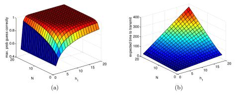
Fig. 2. Analysing security/performance of the NRL pump: (a) Maximum probability of covert channel success; (b) Maximum expected transmission time.
