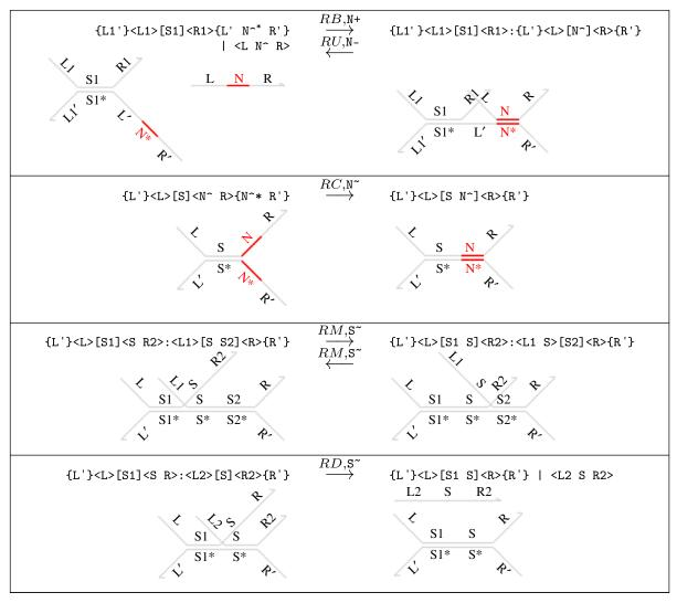
Figure 16. Elementary reduction rules of the DSD programming language. We let S<sup>~</sup> denote the migration rate of a domain sequence S and fst (S) denote its first domain. We also let N+ and N - denote the binding and unbinding rates, respectively, of a toehold N<sup>\(\circ\)</sup>. We assume that  $fst(R2) \neq fst(S2)$  for rule (RM). This ensures that branch migration is maximal along a given sequence and that rules (RM) and (RD) are mutually exclusive. (Online version in colour.)
