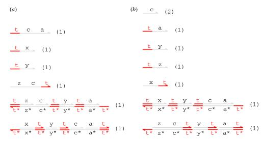
Figure 11. (a) Initial species and (b) expected final species for the alternative catalyst gate C\_NoGC (1, x, y, z). Note that this gate does not perform the additional garbage collection reactions that produced the completely inert structures seen in figure 10. (Online version in colour.)
